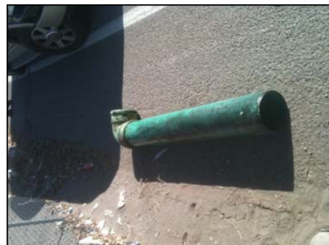
10" diameter pipe removed from old sewer interceptor
